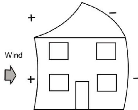
**Figure 7.** a 20pa pressure difference between inside and out (equivalent to a velocity of 2.5m/s) the air flow through 300mm of insulation would result in a 35% reduction in thermal performance. Bankvall [1978].
